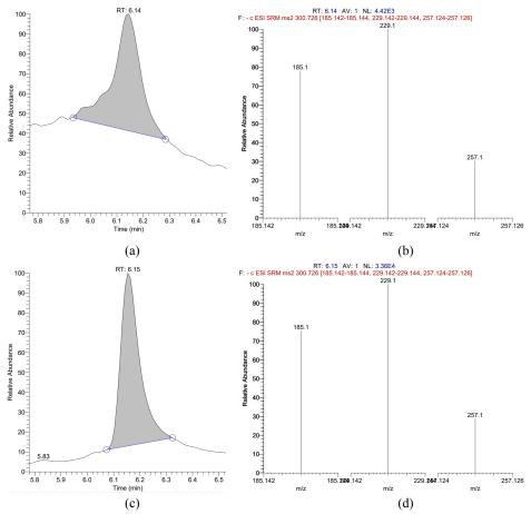
Figure 2. UHPLC-MS/MS chromatograms and electrospray product ion mass spectra of ellagic acid in longan aril and seed extracts. (a, c) UHPLC-MS/MS chromatogram of ellagic acid in longan (a) aril extract and (c) seed extract. (b, d) Electrospray product ion mass spectra of ellagic acid in longan (b) aril extract and (d) seed extract.
