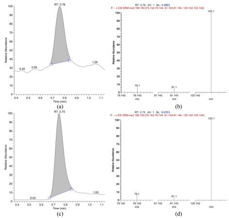
Figure 1. UHPLC-MS/MS chromatograms and electrospray product ion mass spectra of gallic acid in longan aril and seed extracts. (a, c) UHPLC-MS/MS chromatogram of gallic acid in longan (a) aril extract and (c) seed extract. (b, d) Electrospray product ion mass spectra of gallic acid in longan (b) aril extract and (d) seed extract.
